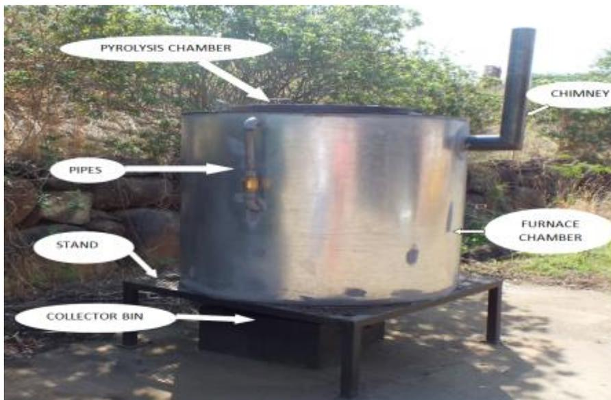
Figure 3 - Biochar manufacturing unit
