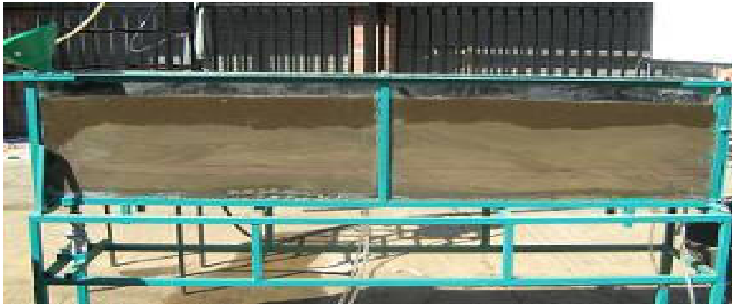
Figure 4: Wetting pattern of furrow irrigation in sand and clay soils
