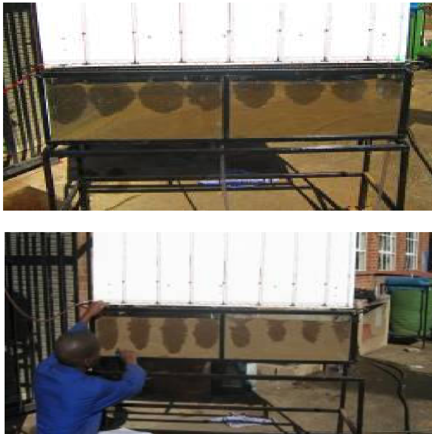
Figure 3: Wetting pattern of drip irrigation in clay and sand soils
